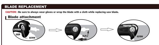
Insert the blade into the handle until the slit in the blade is completely covered, then screw to fix the blade firmly.
